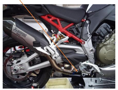
4. Use the supplied hook as shown in the photo to anchor the support spring.
