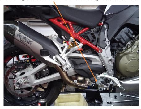
2. Respect the tightening torque of this screw, it is not the swingarm axis, it only acts as a support for the chassis trim
