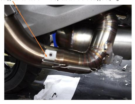
5. If your multistrada has a center stand, you need to remove the center stand before installing the catalyst suppressor. We recommend disassembling all the stand fasteners before the springs.
